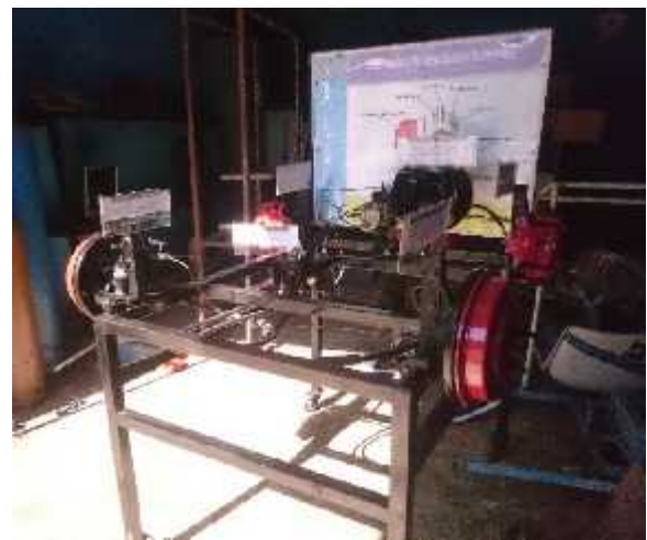
Gambar 2. Model system Pengereman ABS
